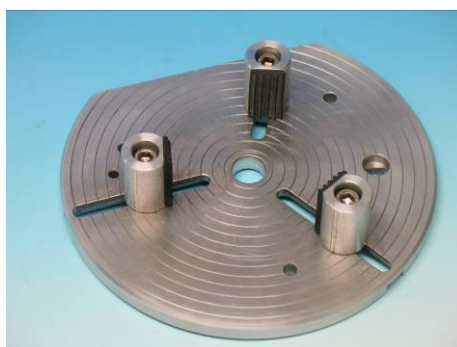
Fig. 1: Universal container holder with three adjustable clamps (left), Fig. 2: Universal clamp holder with a peanut butter glass jar mounted on the HAAKE MARS with a vane rotor FL22 (right)
