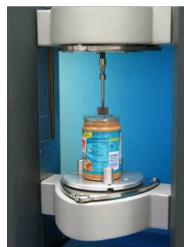
Fig. 1: Universal container holder with three adjustable clamps (left), Fig. 2: Universal clamp holder with a peanut butter glass jar mounted on the HAAKE MARS with a vane rotor FL22 (right)
